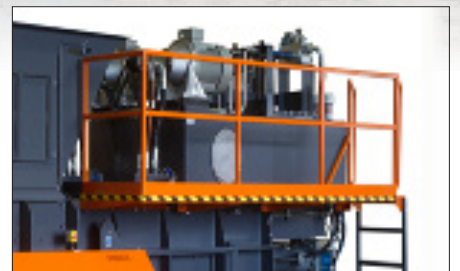
POWER PACK ACCESS GANTRY
